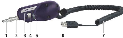
Fig. 20 P5000i Digital Probe components
