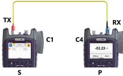
Fig. 25 One jumper reference - unidirectional
