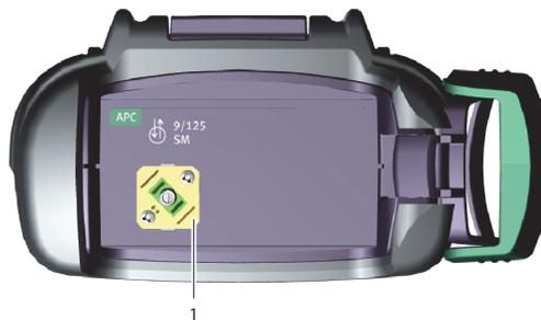
Fig. 3 Connector panel
