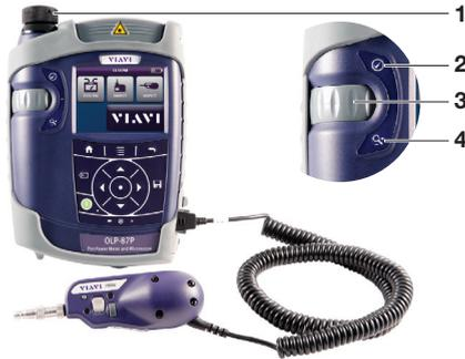
Fig. 19 Patch cord microscope components
