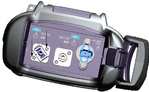
Fig. 7 Mounting the SENKO test adapter
