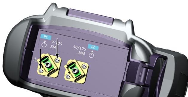
Fig. 9 Mounting the SENKO test adapter
