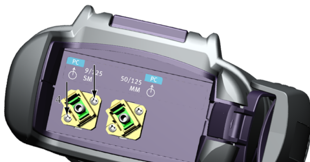
Fig. 9 Mounting the SENKO test adapter
