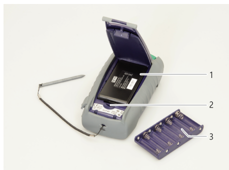
Fig. 5 Replacing the batteries
